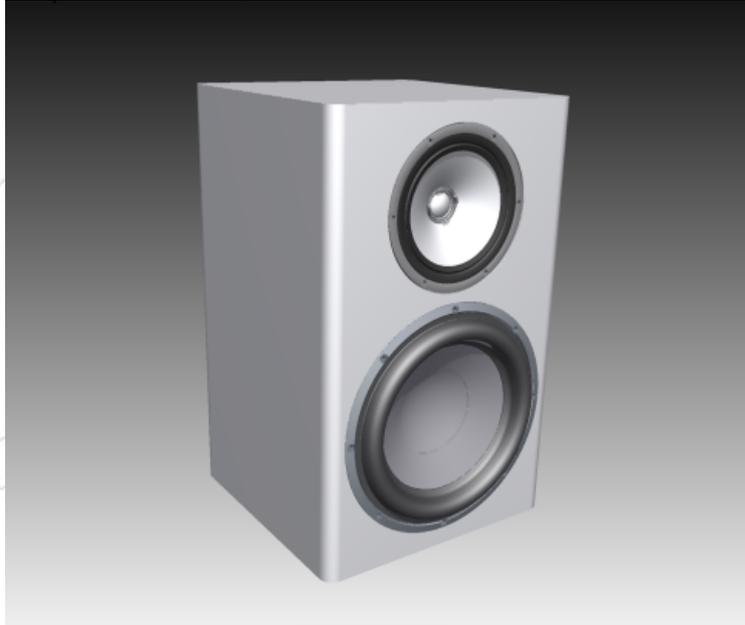
The SEAS KingRO4Y is a 3-way loudspeaker kit, using a 26 cm aluminium cone subwoofer and an 18cm midrange coaxial. The coaxial unit uses a magnesium/aluminium-alloy cone for both the midrange and dome tweeter. All are housed in a compact closed box enclosure and powered by the Hypex PSC2.400 DSP amplifier.
