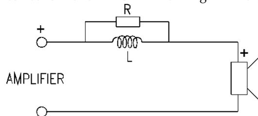
A 0.5 mH inductor (L) will start rolling off from approx. 2 kHz. A larger inductor will be effective at a lower frequency. Use a high quality air core inductor with low DC resistance. The parallel resistor (R) controls the high frequency attenuation. A larger resistance results in more attenuation. Resistors between 1 and 5 Ohms should cover most needs, but other values can be tried without risk of damage. A metal film resistor of 5 watts or higher is recommended.
