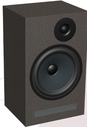
The SEAS A26 is a 2-way loudspeaker kit, using a 26 cm paper cone woofer and a 35 mm textile dome tweeter, in a compact 28 liter aperiodic enclosure. Carefully designed drivers with complementary response characteristics allow for a crossover network using only two components.
