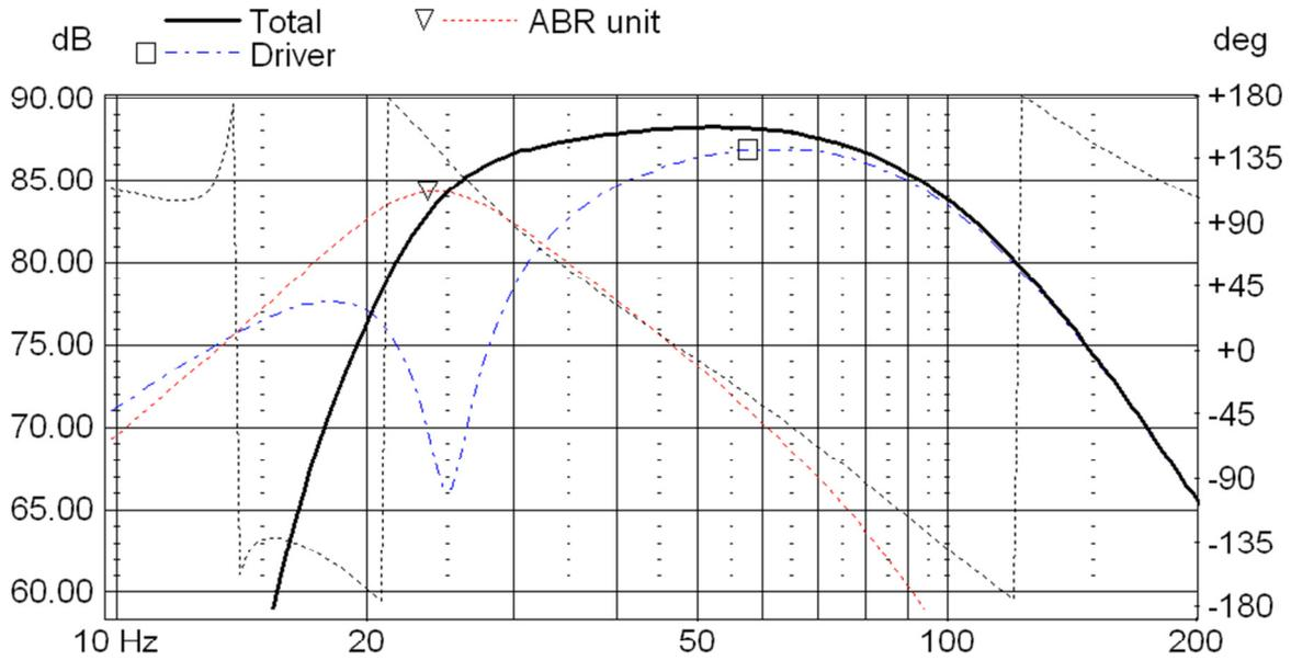
In the case of a bass-reflex enclosure of the same cabinet size, a port with an ID of 7cm would have to be 38cm long in order to achieve a Helmholtz resonance at 25Hz. This leaves only 1cm to the back wall if a straight tube is used, so we don't recommend this.
