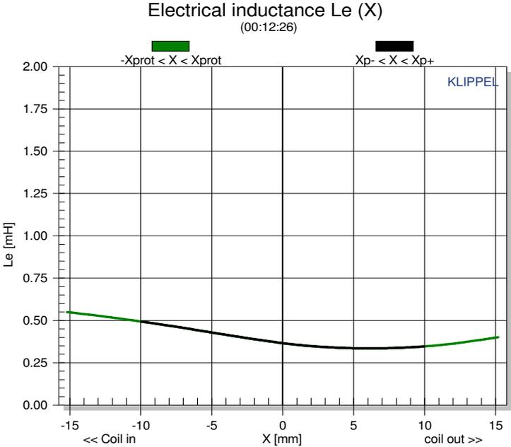
To get the force factor we need to achieve the right T/S parameters, we need an extremely large magnetsystem when using a 2-layer voice coil. The driver is very heavy and must be securely fastened to the enclosure. The Klippel LSI measurements show us that we have a very linear motor. The force factor is very symmetric due to the FEA optimized magnetic circuit, and it has only decreased by 20% when the voice coil has been displaced by 14mm in one direction.
