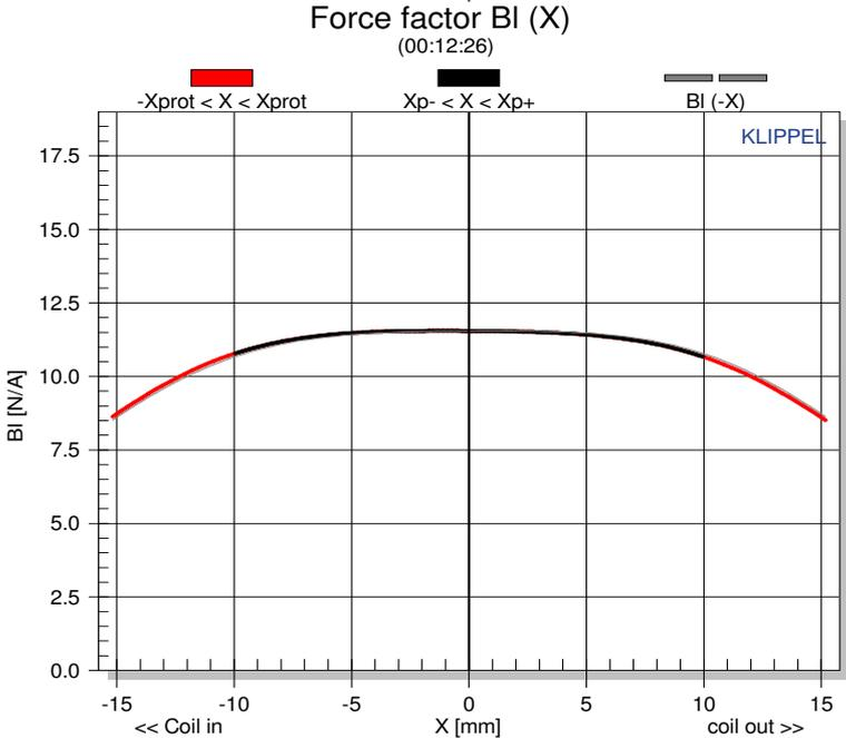
The suspension components have also been optimized by the use of modern FEA software to allow for very long excursion, while keeping the voice coil centered in the air-gap. Again, the Klippel LSI measurements confirm that the simulation has been successfully converted to a really good performing product.
