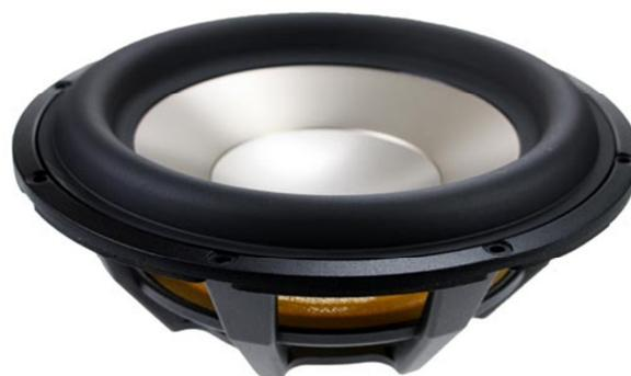
The simulated half-space response of the L26ROY with the SL26R passive radiator in a 40 liter box predicts a resonance frequency for the passive at 25Hz. With a low-pass filter commonly used in a subwoofer application, the -3dB point for the system is at 26Hz, and -10dB is at 21Hz.
